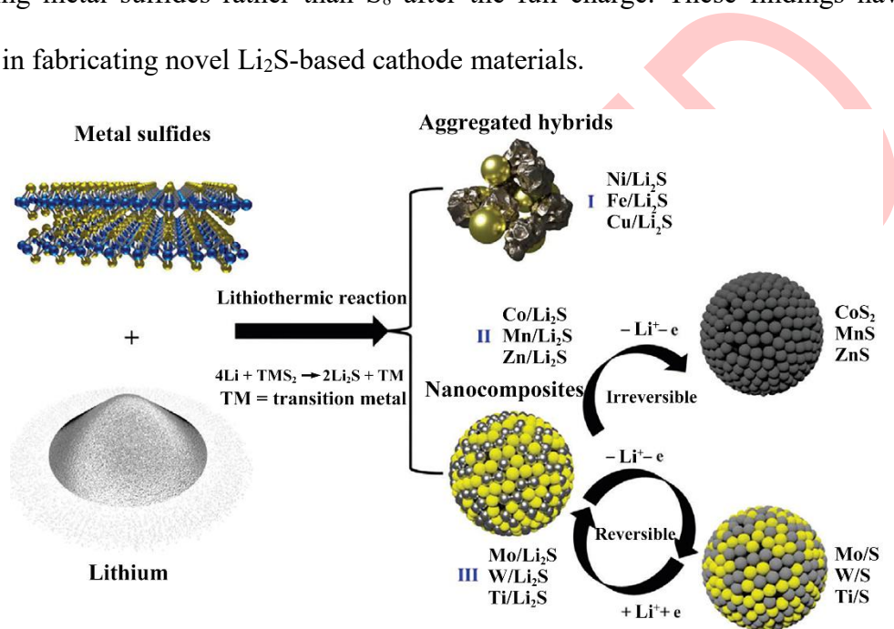
8 9 Fig. 4 Schematic of Li 2 S/TMs synthesis and proposed electrochemical reaction mechanism. 10 Reprinted from Xing Z, Tan G, Yuan Y, et al., Adv Mater , 2020, 32(31): 2002403, Copyright 2020, 11 with permission from Wiley-VCH Verlag GmbH & Co. KGaA [54] .
