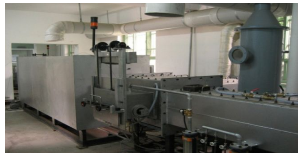
图 7 碱活化制备活性炭连续式中试线 Fig. 7 Photograph showing a pilot line for continuous scale production of activated carbon by alkali activation
