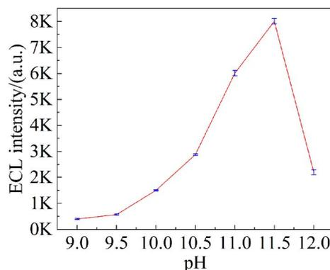
**Figure 4** Effect of pH on ECL intensity using  $0.1 \text{ mol}\cdot\text{L}^{-1}$  CBS,  $0.5 \text{ mmol}\cdot\text{L}^{-1}$  SA, and  $100 \mu\text{mol}\cdot\text{L}^{-1}$  luminol. PMT was biased at 900 V. (color on line)
