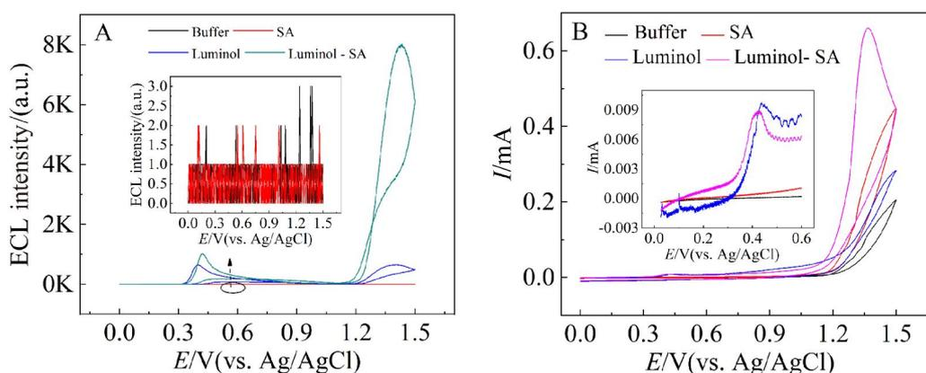
**Figure 1** (A) ECL signal vs potential profile and (B) cyclic voltammograms in CBS ( $0.1 \text{ mol}\cdot\text{L}^{-1}$ , pH 11.5): Buffer solution alone (black color),  $0.5 \text{ mmol}\cdot\text{L}^{-1}$  SA (Red color),  $100 \mu\text{mol}\cdot\text{L}^{-1}$  luminol (blue color), a mixture of  $0.5 \text{ mmol}\cdot\text{L}^{-1}$  SA and  $100 \mu\text{mol}\cdot\text{L}^{-1}$  luminol (green color); scan rate at  $100 \text{ mV}\cdot\text{s}^{-1}$ , PMT at 900 V (color on line)
