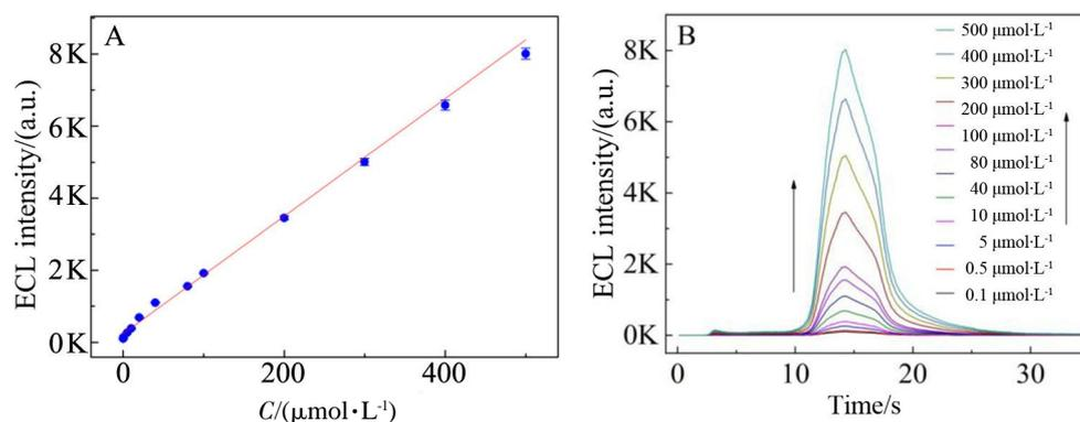
**Figure 5** (A) SA calibration curve and (B) ECL intensity vs. time at different concentrations of SA. 100  $\mu\text{mol}\cdot\text{L}^{-1}$  luminol in 0.1  $\text{mol}\cdot\text{L}^{-1}$  pH 11.5 CBS. (color on line)
