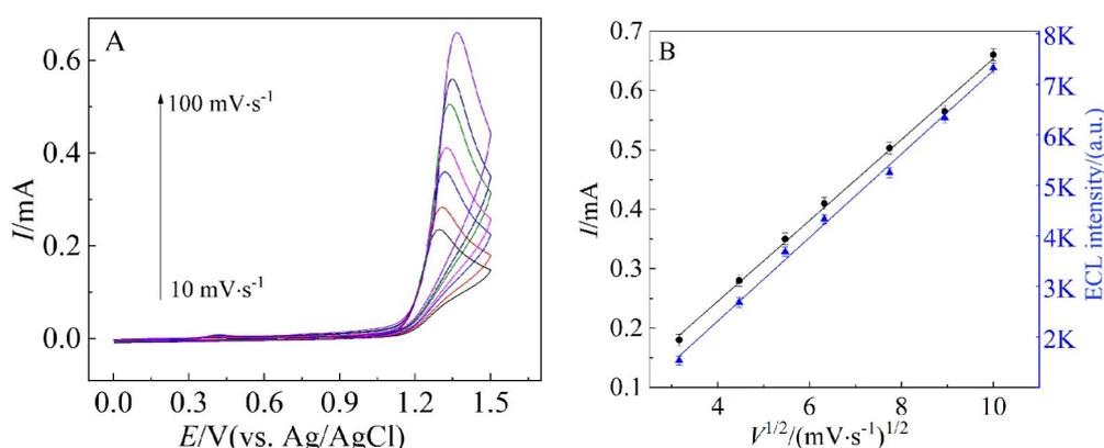
**Figure 2** (A) Effect of scan rate on cyclic voltammograms and (B) variations of peak current and ECL intensity with the square root of scan rate ( $v^{1/2}$ ) in  $0.5 \text{ mmol}\cdot\text{L}^{-1}$  SA and  $100 \mu\text{mol}\cdot\text{L}^{-1}$  luminol (color on line)
