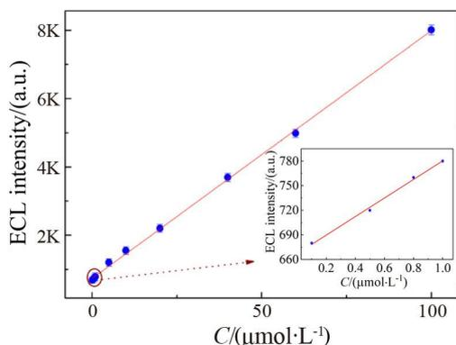
**Figure 6** ECL intensity vs. concentration of luminol. 0.5  $\text{mmol}\cdot\text{L}^{-1}$  SA in 0.1  $\text{mol}\cdot\text{L}^{-1}$  pH 11.5 CBS. The inset shows the plot at low concentration ( $\leq 1.0 \mu\text{mol}\cdot\text{L}^{-1}$ ). (color on line)
