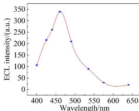
**Figure 3** Emission spectrum of  $100 \mu\text{mol}\cdot\text{L}^{-1}$  luminol and  $0.5 \text{ mmol}\cdot\text{L}^{-1}$  SA system.  $0.1 \text{ mol}\cdot\text{L}^{-1}$  CBS of  $\text{pH} = 11.5$  and PMT was biased at 900 V. (color on line)
