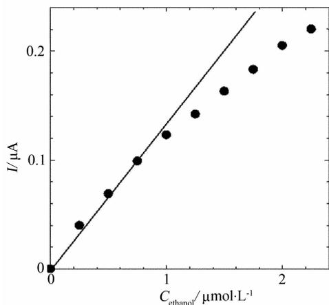
Fig. 4 The plot of the steady-state current against ethanol concentration using the data obtained from Fig. 3
