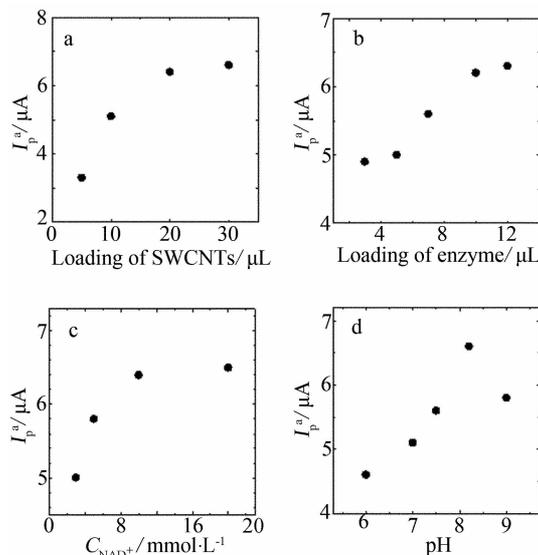
Fig. 2 Effects of experimental parameters on the electrocatalytic response of the ADH/PPS-SWCNT/EPPG electrode for the ethanol oxidation in  $0.05 \text{ mol} \cdot \text{L}^{-1}$  TBS (pH 8.2) in the presence of  $20 \text{ mmol} \cdot \text{L}^{-1}$  ethanol
