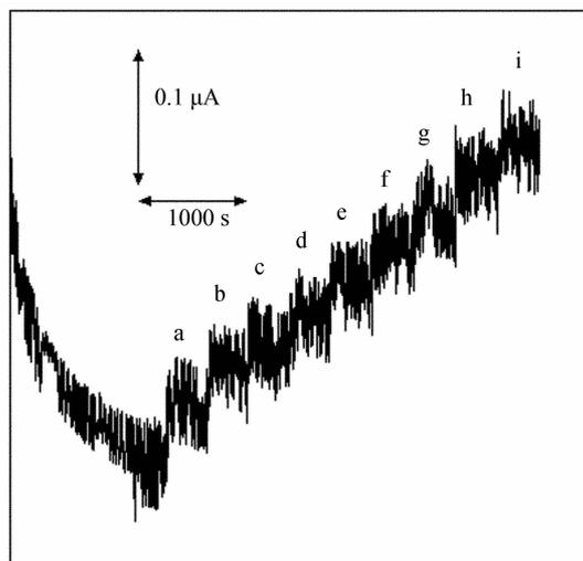
Fig. 3 Current ~ time response of the ADH/PPS-SWCNT/EPPG electrode for the successive addition of  $250 \mu\text{mol} \cdot \text{L}^{-1}$  ethanol at  $0.2 \text{ V}$  in  $0.05 \text{ mol} \cdot \text{L}^{-1}$  TBS (pH  $8.2$ ) containing  $10 \text{ mmol} \cdot \text{L}^{-1}$   $\text{NAD}^+$   $C_{\text{ethanol}}/\mu\text{mol} \cdot \text{L}^{-1}$ : a.  $250$ , b.  $500$ , c.  $750$ , d.  $1000$ , e.  $1250$ , f.  $1500$ , g.  $1750$ , h.  $2000$ , i.  $2250$
