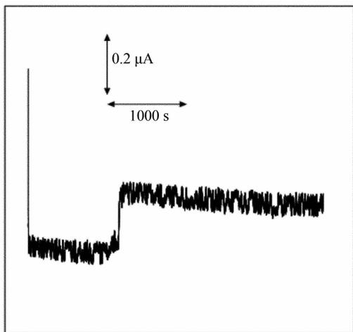
Fig. 5 A continuous recording of the current response of the ADH/PPS-SWCNT/EPPG electrode in  $0.05 \text{ mol} \cdot \text{L}^{-1}$  TBS (pH 8.2) containing  $10 \text{ mmol} \cdot \text{L}^{-1}$   $\text{NAD}^+$  and  $1.0 \text{ mmol} \cdot \text{L}^{-1}$  ethanol at an operating potential of  $0.2 \text{ V}$  other experimental conditions are the same as in Fig. 3
