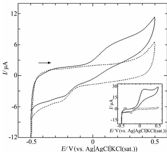
Fig. 1 CVs obtained at the ADH/PPS-SWCNT/EPPG electrode in  $0.05 \text{ mol} \cdot \text{L}^{-1}$  TBS (pH 8.2) containing  $10 \text{ mmol} \cdot \text{L}^{-1}$   $\text{NAD}^+$  in the presence (—) and absence (---) of  $20 \text{ mmol} \cdot \text{L}^{-1}$  ethanol
