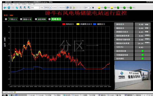
图 7 储能电站接受调度参与电网调峰的情况 Fig. 7 Peak shaving response with VFB energy storage system ordered by grid dispatch center
