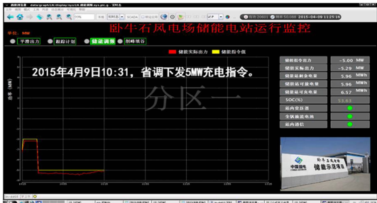
图 6 储能电站接受调度参与调频的响应情况 Fig. 6 Frequency regulation response with VFB energy storage system ordered by grid dispatch center
