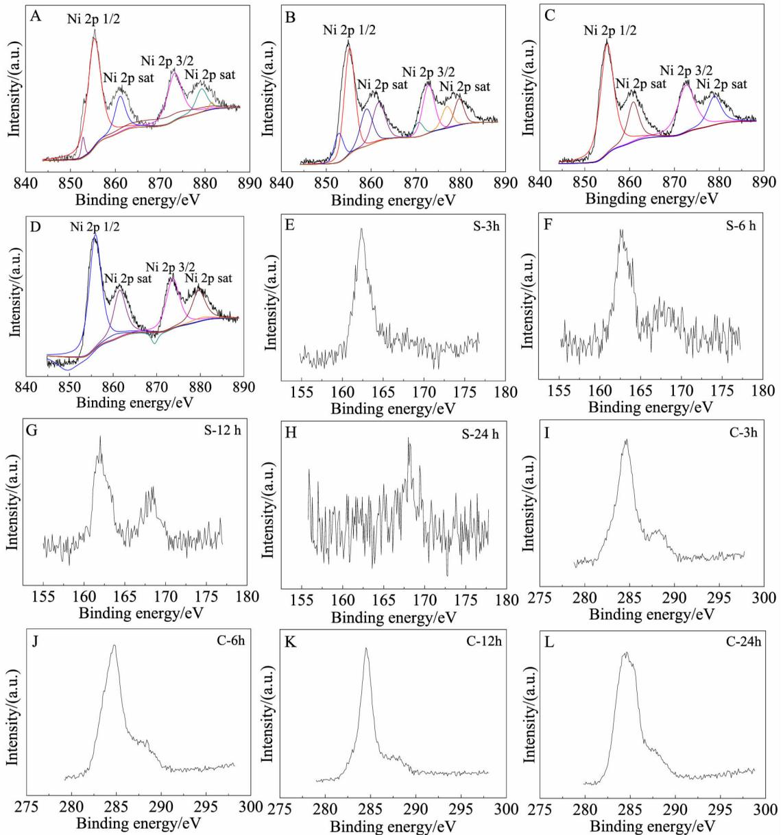
Fig. 5 XPS spectra of Ni 2p (A-D), S2p (E-H) and C1s (I-L) the for  $\text{Ni}_3\text{S}_2/3\text{DG}$  composite prepared with various reaction time
