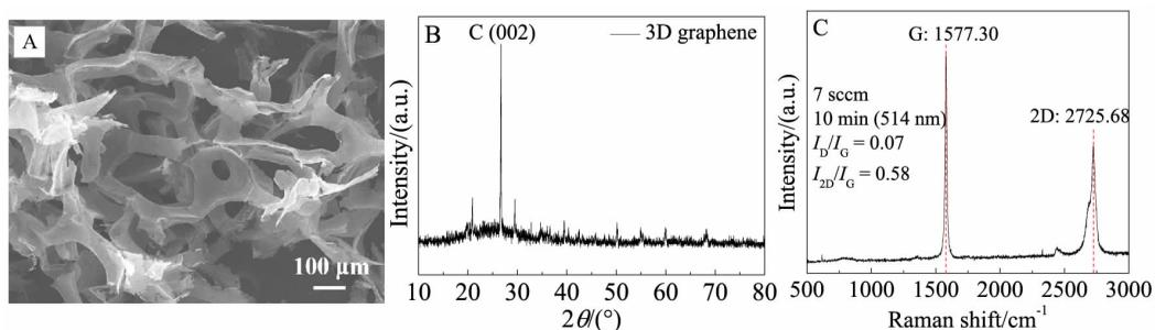
Fig. 1 SEM image (A), XRD pattern (B), and Raman spectrum (C) of 3DG
