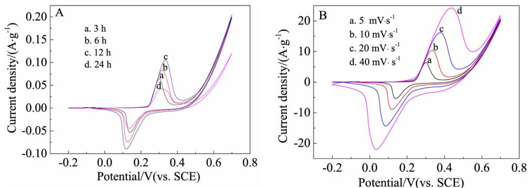
Fig. 6 A. Cyclic voltammograms of composite electrodes measured at a scan rate of  $5 \text{ mV} \cdot \text{s}^{-1}$ ; B. Cyclic voltammograms of  $\text{Ni}_3\text{S}_2/3\text{DG}$ -12 h electrode at various scan rates
