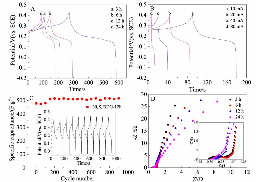
Fig. 7 Electrochemical performances of the composite electrodes
