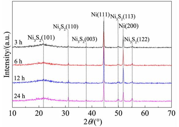
Fig. 3 XRD patterns of Ni<sub>3</sub>S<sub>2</sub>/3DG prepared with different reaction time
