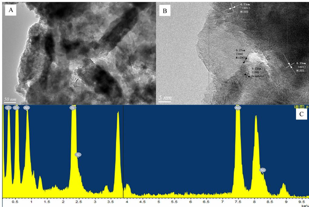
Fig. 4 High resolution TEM image (A), Lattice fringe image (B), and EDS pattern (C) of Ni<sub>3</sub>S<sub>2</sub>/3DG
