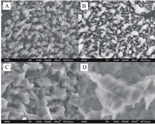
Fig. 2 SEM images of Ni<sub>3</sub>S<sub>2</sub>/3DG prepared with different reaction time
