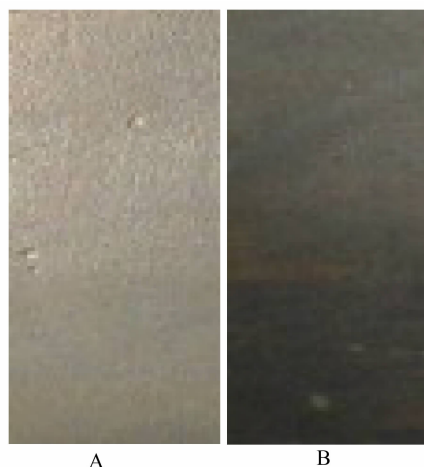
图 7 镍电极氟化反应前(A)后(B)表面照片 Fig. 7 Photographs of Ni electrode before (A) and after (B) the Simons electrochemical fluorination
