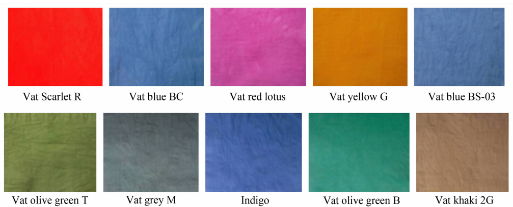
图 5 Fe(III)-草酸-葡萄糖酸钙媒质体系间接电化学还原染色棉织物图片 Fig. 5 Cotton fabric pictures of indirect electrochemical reduction of dyes in Fe(III)-oxalate-calcium gluconate medium
