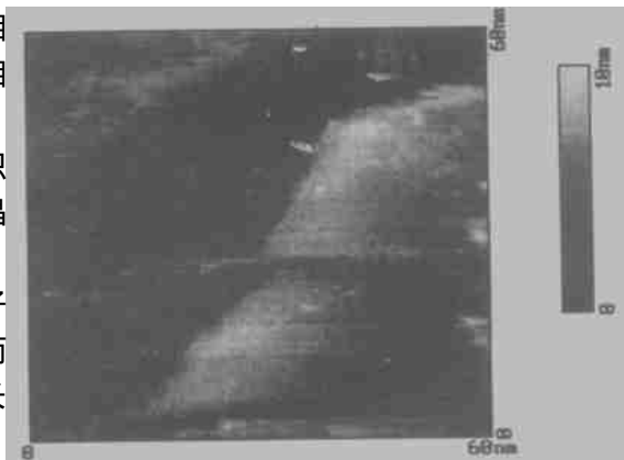
图 4 在 10 mmol/L CuSO 4 溶液中铜电沉积的现场 STM 观察: 当控制电位为 - 300 mV (vs Cu 2+ /Cu) 时, 铜沉积层表面晶粒明显细化 Fig 4 At the potential of - 300 mV (vs Cu 2+ /Cu), the crystal size of deposited layers were somehow smaller ( I_t = 1 \text{ nA} , V_b = 100 \text{ mV} )
