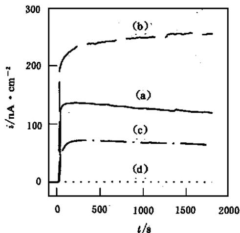
Fig. 4 Galvanic currents between TiN and W measured in 0.01 mol/L KNO<sub>3</sub> solutions at pH 4.0
